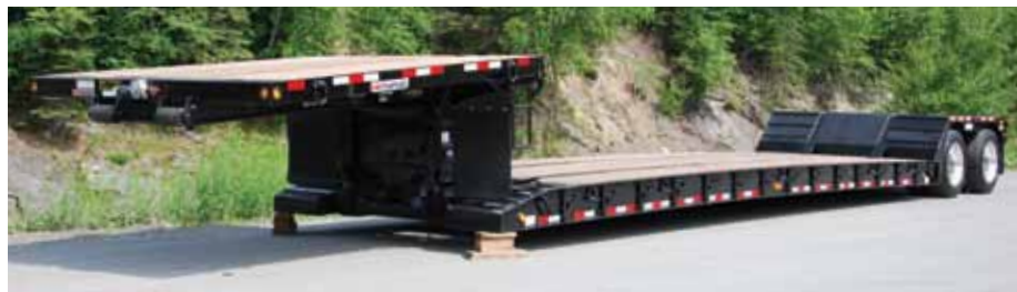
Extensions made of high strength steel
