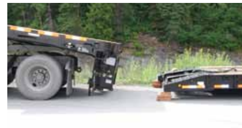
Deck extension with double rollers and air locking pins
