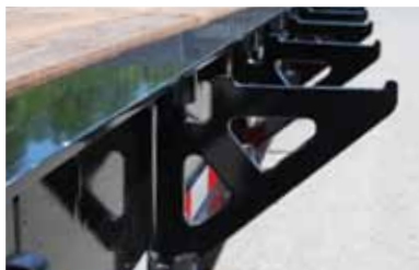
Extensions made of high strength steel
